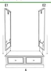
Attach the left hand side (E1) and the right hand side (E2) to the base unit (A).
