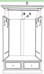
Attach cam bolt (M) x1 to the top (D). Insert cam lock (N) x1 into the upper end of the connecting panel (G).
