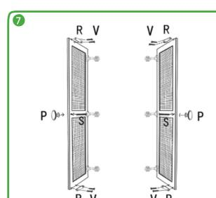
Attach metal plates (R) x4 onto the corners of the doors using screws (V)  $\times 8$ .
