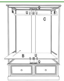
Attach magnetic catches (Q) x4 to the top and bottom of the unit, using screws (U) x8.
