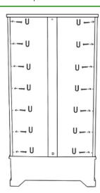
Back panels (H) are screwed inside internal slats of two side panels using screws (U) x14.
