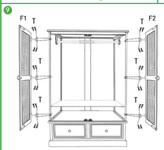
Attach doors (F1&f2) to the unit using screws (T) x24. Level the doors according to the directions of door adjustment.
