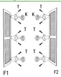
Attach big angle hinges (K) x6 to the doors (F1&F2) using screws (T) x12.
